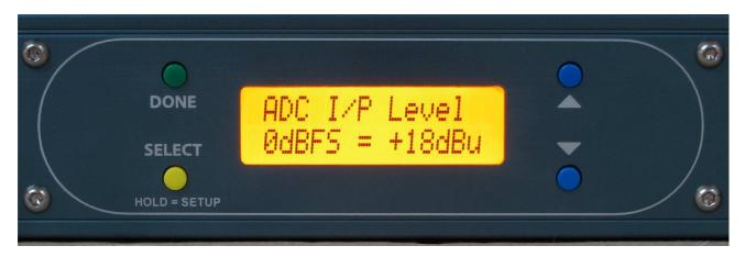
This sets the full scale (0dBFS) digital output level in reference to analogue input level. There are 4 options of 0dBFS equalling:
