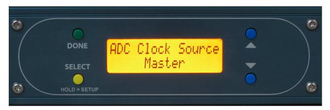
This control sets what clock source is used as a reference for the ADC. The digital output will be locked to the selected source. There are 4 options.
