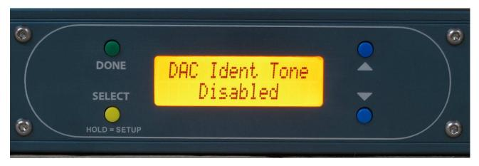
Turning on the DAC Ident tone (enabling it) adds a 1kHz tone @ 0dBu to the analogue output. This can be useful for fault finding.
