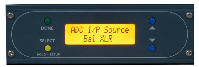
This sets which analogue input source is routed to the AD converter. There are 2 choices:
