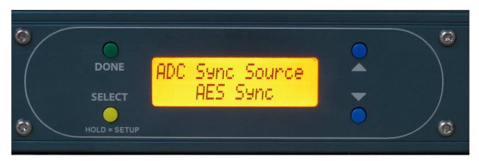
This sets which of the 3 possible external reference clock sources the device should use.
