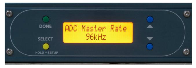
This sets the output sample frequency of the internal clock. There are 6 options:
