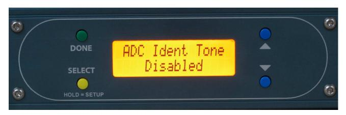
Turning on the ADC Ident tone (enabling it) adds a 1kHz tone @ 0dBu to the digital output. This can be useful for fault finding.
