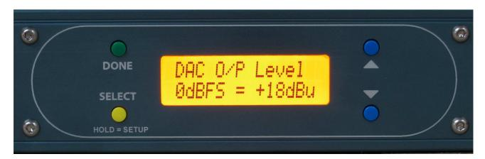
This sets the analogue output level in reference to digital full scale (0dBFS). There are 4 options of 0dBFS equalling:
