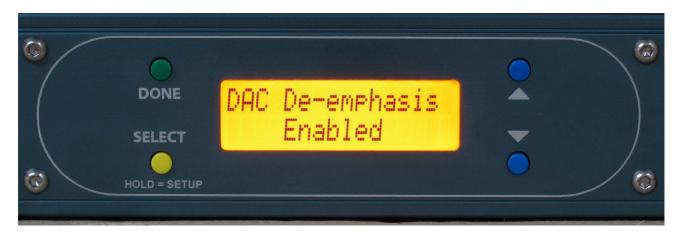
If your digital audio source was originally mastered with pre-emphasis (normally the high frequency boost) then enabling de-emphasis removes this during the D/A process.
