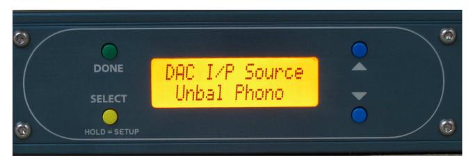
This sets the digital audio input that is fed into the internal D/A converter. There are 3 options:
